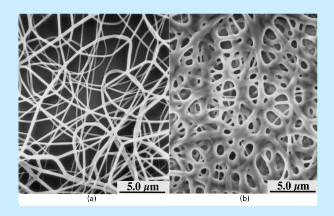
PA fibers, electrode distance 2 cm (a) and 0.5 cm (b)
