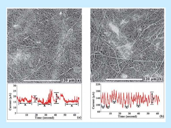
Morphology of fibers as a function of electric current (a) 20 hm.% PU (b) 20 hm.% PU with addition of 1.27% TEAB
