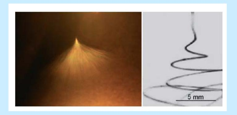
Left: Photograph of a jet of PEO solution during electrospinning.
