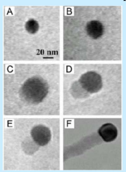
In situ TEM images recorded during the process of nanowire growth. (a) Au nanoclusters in solid state at 500 °C; (b) alloying initiated at 800 °C, at this stage Au exists mostly in solid state; (c) liquid Au/Ge alloy; (d) the nucleation of Ge nanocrystal on the alloy surface; (e) Ge nanocrystal elongates with further Ge condensation and eventually forms a wire (f)
