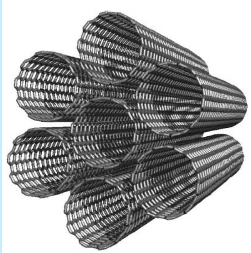
A bundle of (10,10) nanotubes held together with strong  $\pi$ - $\pi$ -stacking interactions
