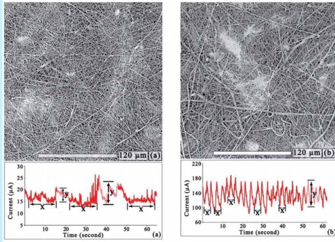
Morphology of fibers as a function of electric current
