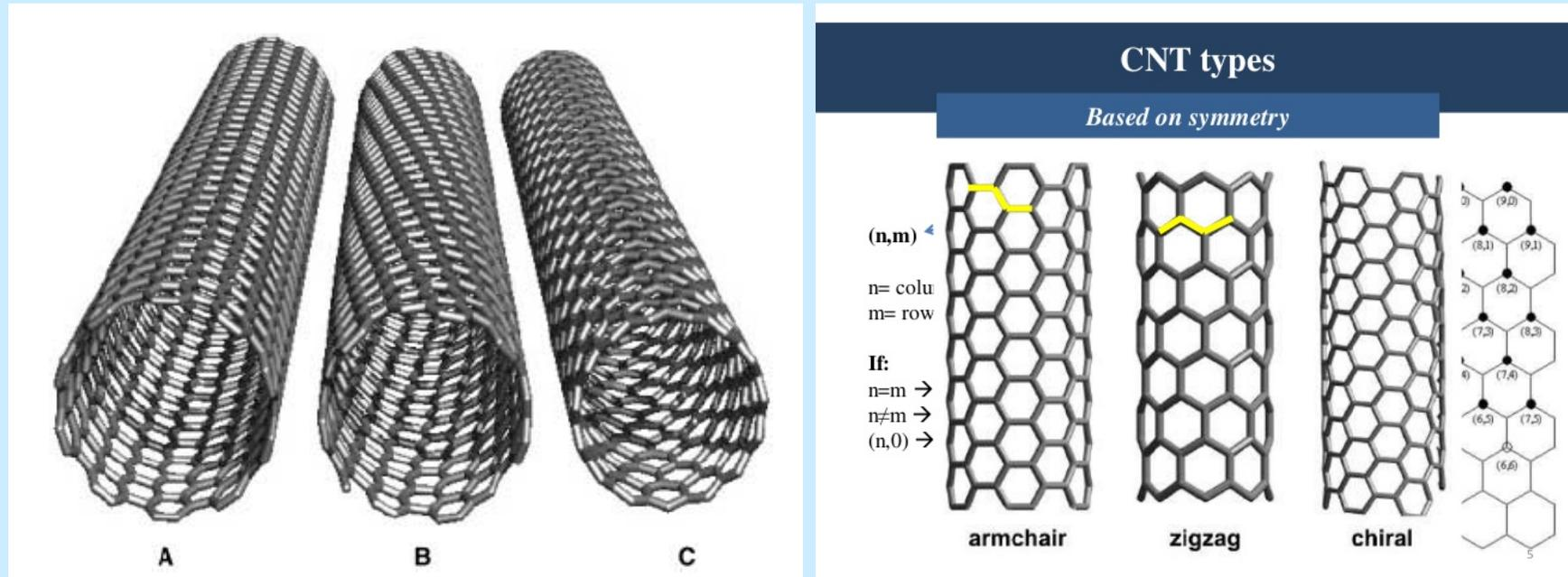
A) Armchair - an achiral metallic conducting (10,10) tube
