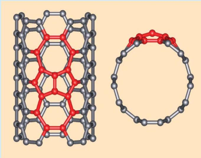
Stone-Wales defect (7-5-5-7 defect)  $\Rightarrow$
