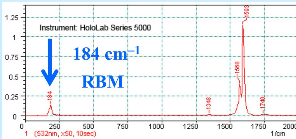
The wavenumber of RBM is inversely proportional to the tube diameter **D**
