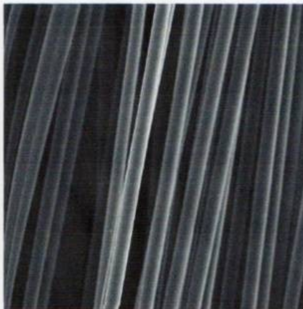
Figure 3. SEM micrograph of reclaimed carbon fiber with 0.22% (w/w) residual resin (500x).
