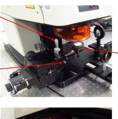
Sample holder with the screws to set the leaning angle of the sample
