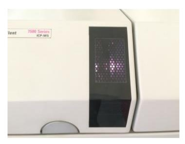
Fig. 7: Ignited plasma in the Mass Spectrometer.
