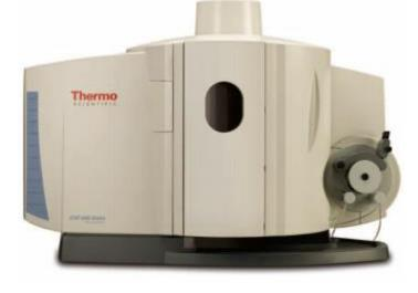
Deretmination of Cu in the sample will be carried out using ICP spectrometer iCAP 6500 Duo (Thermo Scientific). ICP spectrometer contains echelle monochromator with grating with 52,9 grooves per mm. This system offers simultaneous measuring of spectrum in the range 166 –847 nm.
