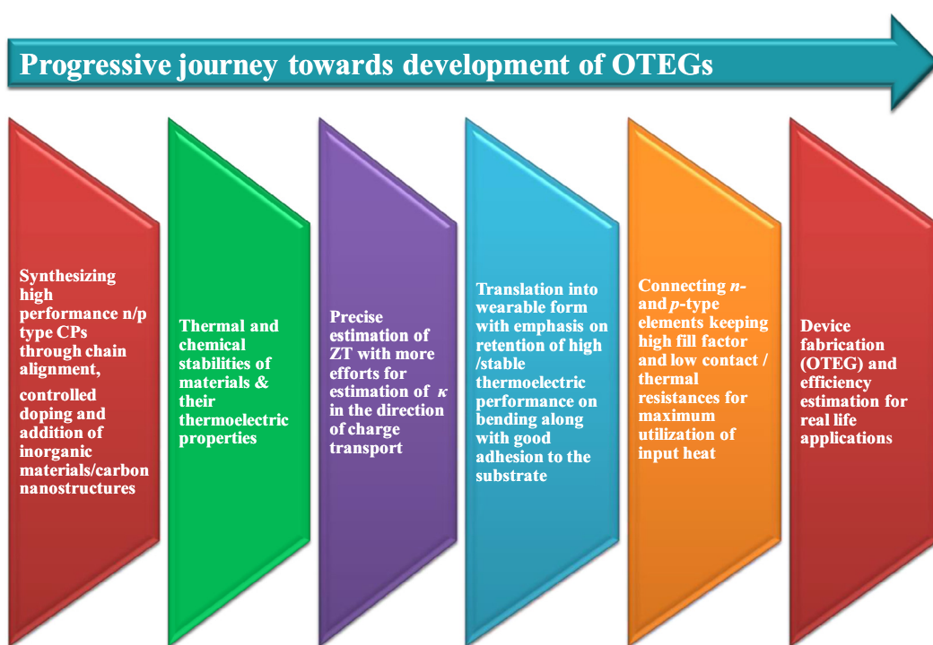
Fig. 33. Schematic revealing various stages of organic thermoelectric power generation.
