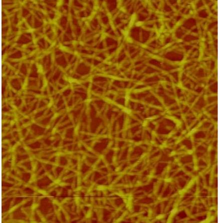
**AFM** height image of carboxymethylated nanocellulose adsorbed on a silica surface. The scanned surface area is 1  $\mu$ m<sup>2</sup> > **FIBRES HAVE DIAMETER approx. 80 – 100 nm**
