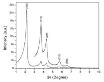
**b**) Now, derive the formula relating the interplanar distance d(100) to the hexagonal mesoporous parameter  $a_0$  and calculate its value.
