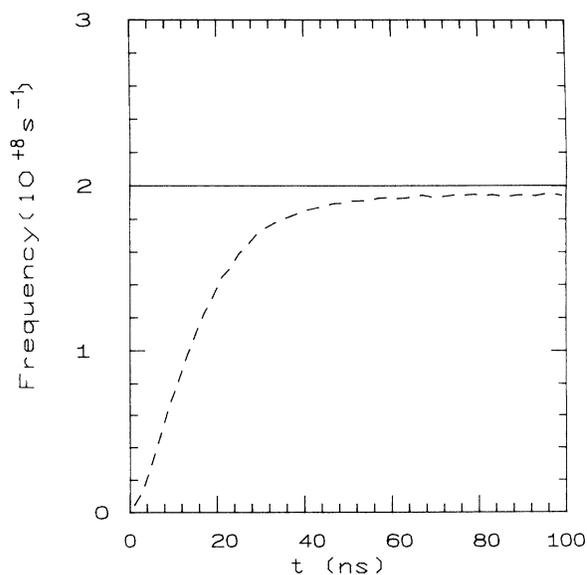
FIG. 8. Electron attachment frequency  $\langle v_{\text{att}} \rangle$  (---) in  $\text{SF}_6$  with fictitious ionization  $v_{\text{fc,ion}}=2 \times 10^8 \text{ s}^{-1}$  (—):  $E/N=10$  Td, 5000 seed electrons, initial electron beam with 2 eV emitted along the forward direction.
