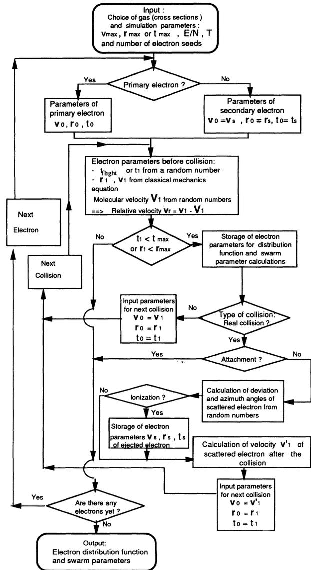
FIG. 1. Flow chart for Monte Carlo simulation of electron swarm motion in a gas under action of an accelerating electric field  $E$  (velocity  $v_{\text{max}}$ , position  $r_{\text{max}}$ , and time  $t_{\text{max}}$  correspond to the possible limits of the simulation domain: see Sec. II for an explanation of the other notations used).
