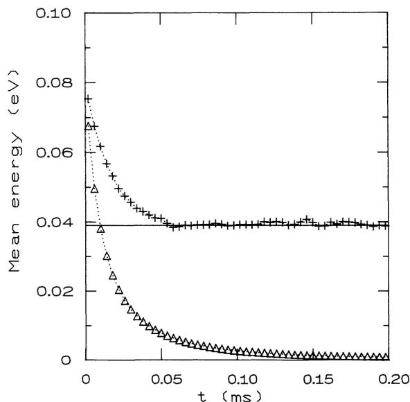
FIG. 3. Zero-field electron mean energy in He for  $p = 1$  Torr,  $T = 300$  K, and an initial electron beam energy  $\epsilon_0 = 0.1$  eV distributed along forward direction: ( $\dots+\dots$ ) including thermal motion of targets and ( $\dots\Delta\dots$ ) target assumed to be at rest.
