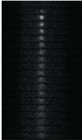
Observation with band scanning Imaging at 420 fps (2.4 ms/frame) Image size: 512 x 32 pixels
