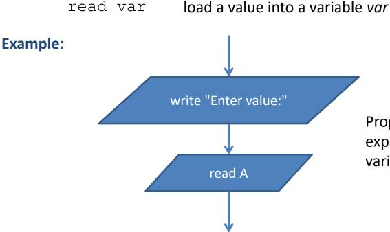
Program writes a query to the user and expects input, which is loaded into the variable A after entering it by the user.
