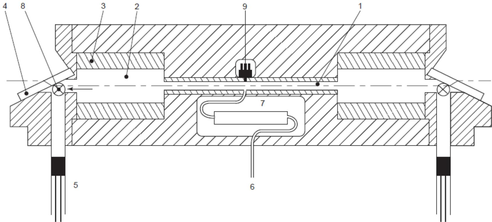
**Figure 4** Resonant photoacoustic cell. 1, resonator; 2, buffer volume (maximum diameter 40 mm, length 50 mm); 3, buffer ring to decrease buffer radius; 4, ZnSe Brewster window; 5, adjustable  $\lambda/4$  notch filter to suppress window signal; 6, inlet gas flow; 7,  $\lambda/2$  notch filter to suppress flow noise; 8, outlet gas flow; 9, Knowless microphone.
