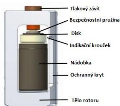
Fig. 6 Segment for decomposition of one sample
