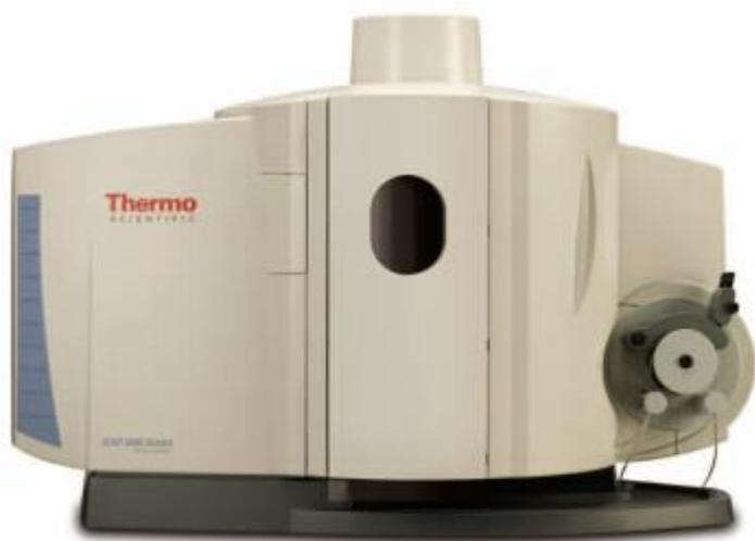
Determination of Cu in the sample will be carried out using ICP spectrometer iCAP 6500 Duo (Thermo Scientific). ICP spectrometer contains echelle monochromator with grating with 52,9 grooves per mm. This system offers simultaneous measuring of spectrum in the range 166 –847 nm.
