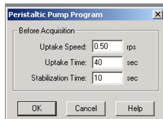
Fig. 6: Program of peristaltic pump.
