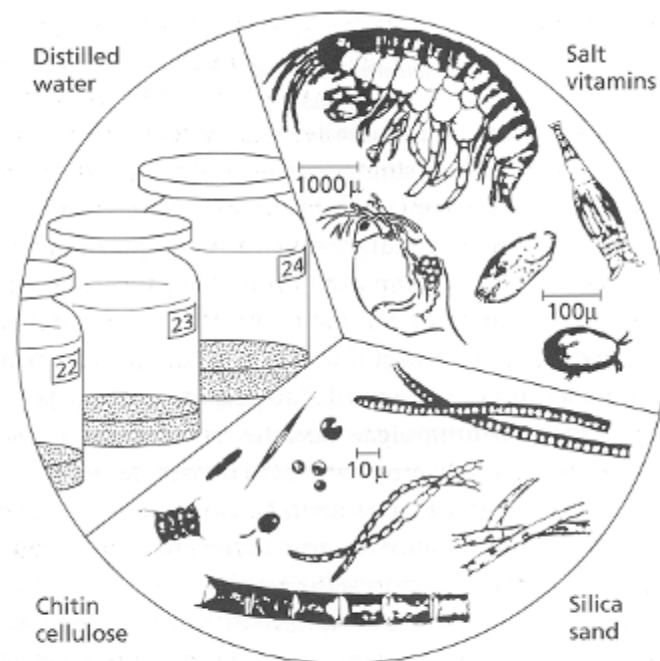
Fig. 5.2 Components of a standardized aquatic microcosm.
