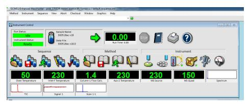
2. Click to **Method** > **Run Method**, fill the sample name and click to **OK and Run Method** button. Wait till window **GC Aquisition** for valve switching will occur.
