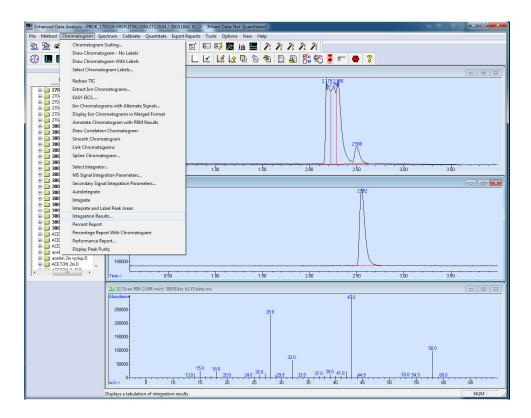
10. Click (right-click) to any peak in mass spectrometry (TIC) chromatogram (upper). Mass spectrum of related compound will occur. Then click to Spectrum > NIST Search in the upper bar of the Data Analysis window and most probable reference spectrum will be found in a new NIST window.
