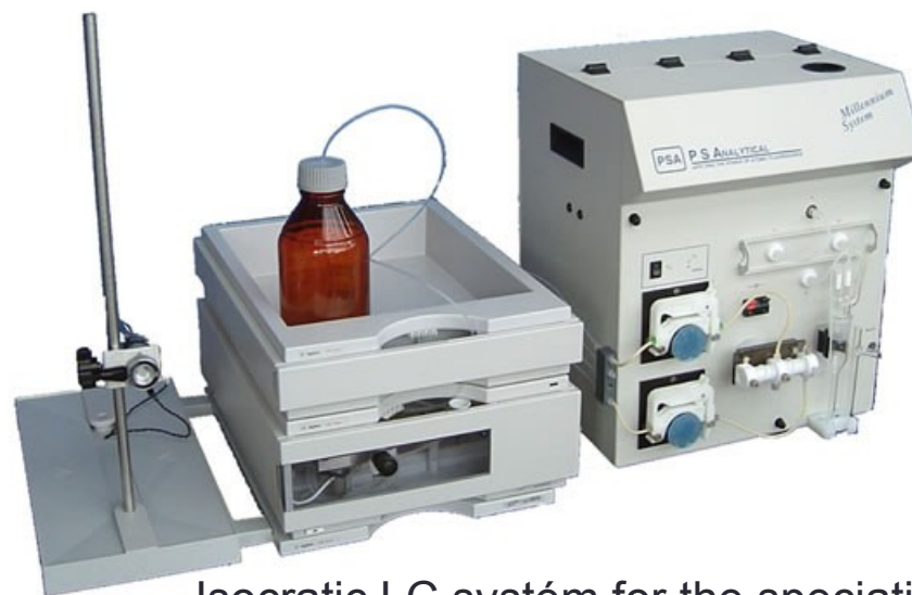
Isocratic LC system for the speciation of Selenium
