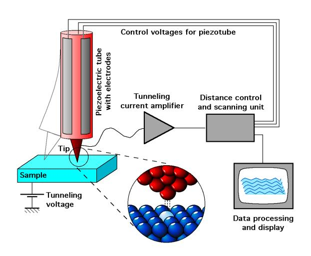
A tip is scanned over a surface at a distance of a few atomic diameters in a point-by-point and line-by-line fashion. At each point the tunneling current between the tip and the surface is measured. The tunneling current decreases exponentially with increasing distance and thus, through the use of a feedback loop, the vertical position of the tip can be adjusted to a constant distance from the surface.
