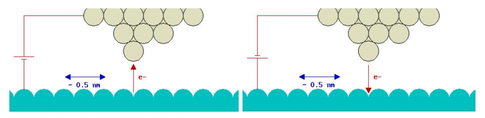
If the sample is biased -ve with respect to the tip, then electrons will flow from the surface to the tip as shown on the left, whilst if the sample is biased +ve with respect to the tip, then electrons will flow from the tip to the surface as shown on the right.
