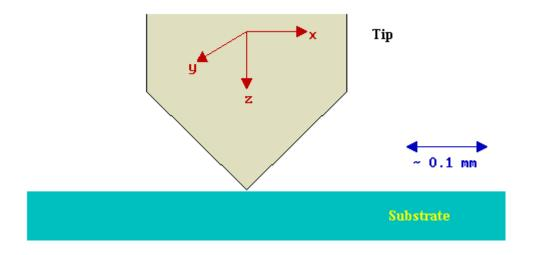
STM - is the *tunnelling current* between a metallic tip and a conducting substrate which are in very close proximity but not actually in physical contact.
