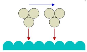
If the tip is scanned at what is nominally a constant height above the surface, then there is actually a periodic variation in the separation distance between the tip and surface atoms. At one point the tip will be directly above a surface atom and the tunnelling current will be large whilst at other points the tip will be above hollow sites on the surface and the tunnelling current will be much smaller.
