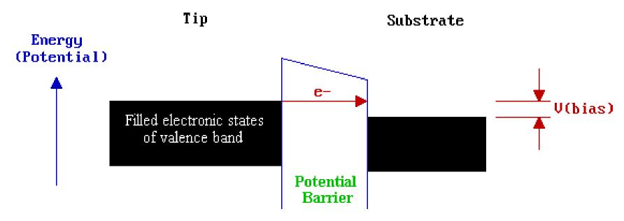
In this model, the probability of tunnelling is exponentially-dependent upon the distance of separation between the tip and surface: the tunnelling current is therefore a very sensitive probe of this separation.
