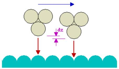
The image is then formed by plotting the tip height (strictly, the voltage applied to the z-piezo) v's the lateral tip position.
