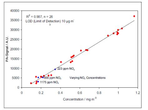
Figure 5. Calibration curve of the PASS system vs thermochemical analysis.
