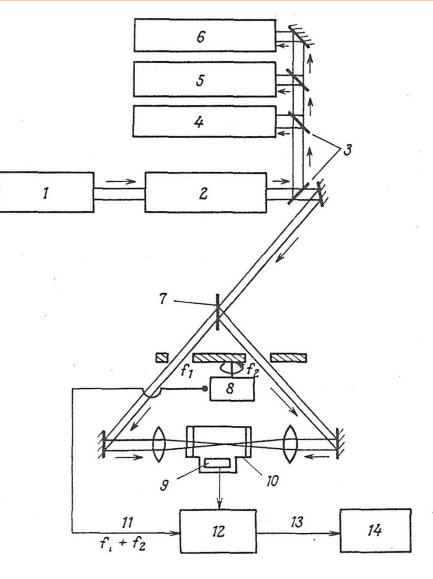
The frequency equal to the sum f1 + f2 will be generated only if both opposite beams saturate the same particles, ie particles at zero velocity with respect to the beams.
