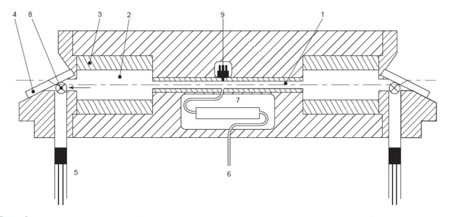
**Figure 4** Resonant photoacoustic cell. 1, resonator; 2, buffer volume (maximum diameter 40 mm, length 50 mm); 3, buffer ring to decrease buffer radius; 4, ZnSe Brewster window; 5, adjustable  $\lambda/4$  notch filter to suppress window signal; 6, inlet gas flow; 7,  $\lambda/2$  notch filter to suppress flow noise; 8, outlet gas flow; 9, Knowless microphone.
