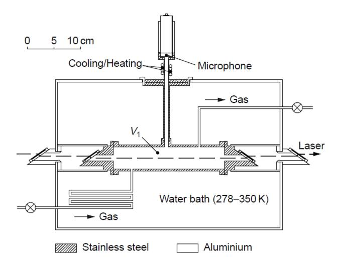
Photoacoustic cell applied for temperature-dependent investigations on fatty acids. The temperature of the water bath was varied between 278 and 350K with a cold finger and two immersion heaters, while the temperature of the microphone was kept constant with a cooling/heating device.
