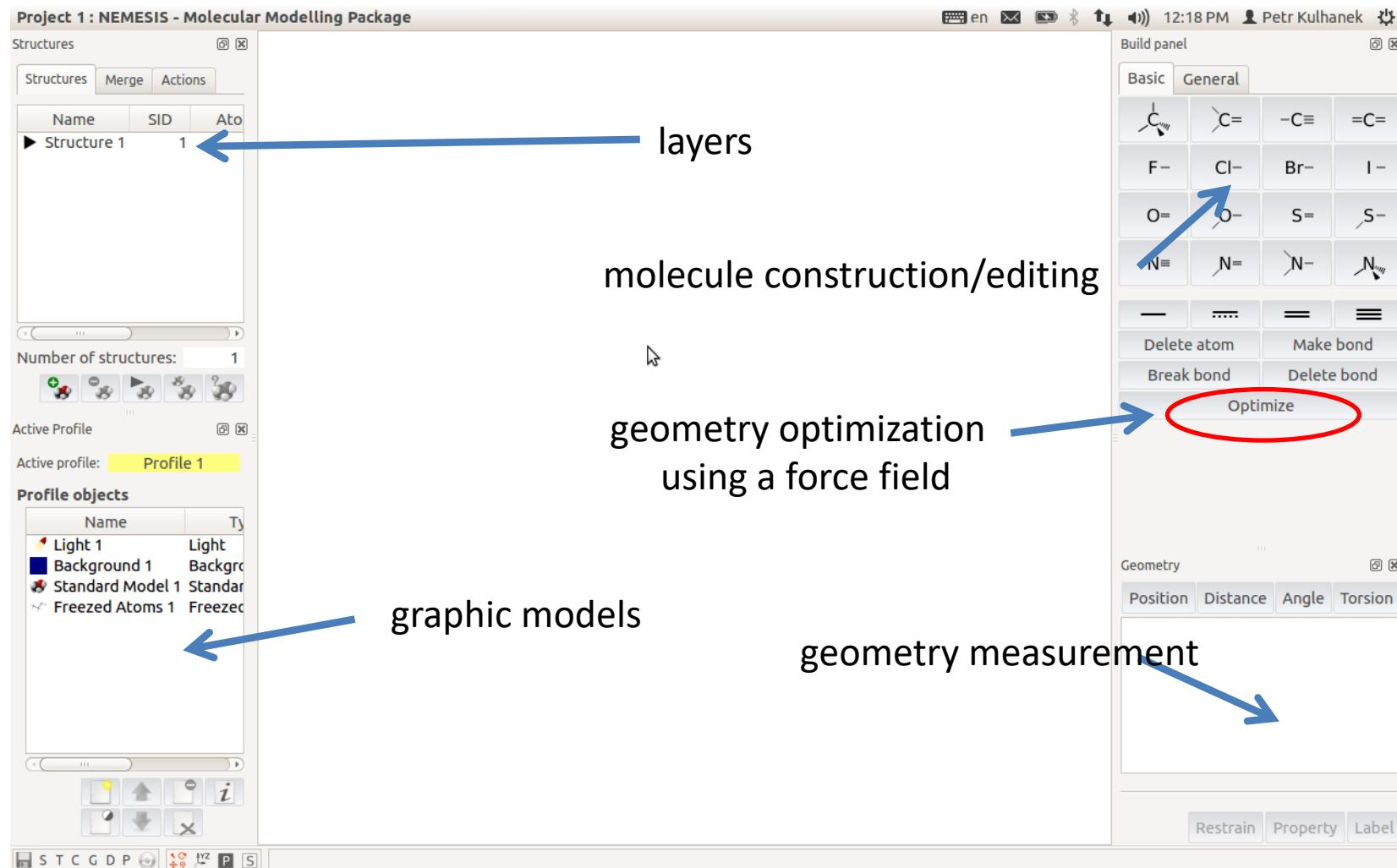
Force field settings for optimization: menu Geometry-> Optimizer Setup
