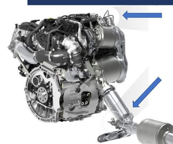
Injection of AdBlue (32,5 % solution of urea in distilled water)
