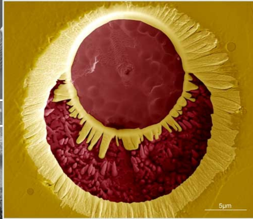
FIB-cut in steel wafer by 1nA to 1 μm milling 002 steel wafer imaged with a plasma FIB
