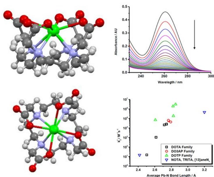
Figure 1 – a) calculated structure of the Pb(II)-DOTA complex, b) dissociation of the Pb(II)-DOTA complex in 1M HClO<sub>4</sub>, and c) graph showing the correlation between the formation rate constant  $k_f^2$  and the average Pb-N bond length for all investigated complexes.
