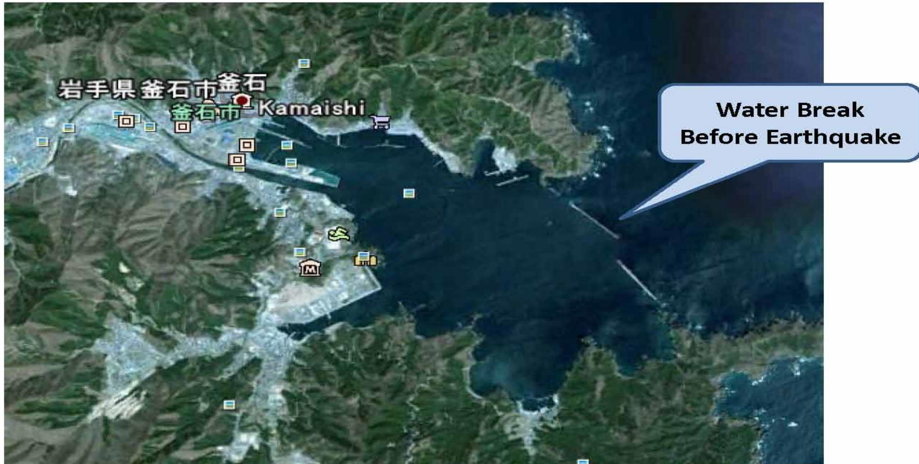
Fig.4a The Deepest Water Break against Tsunami in Kamaishi Bay. Iwate Prefecture
