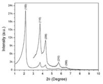
**b)** Now, derive the formula relating the interplanar distance d(100) to the hexagonal mesoporous parameter  $a_0$  and calculate its value.
