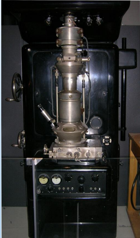
Figure 1.1. The electron microscope built by Ruska and Knoll in Berlin in the early 1930s.
