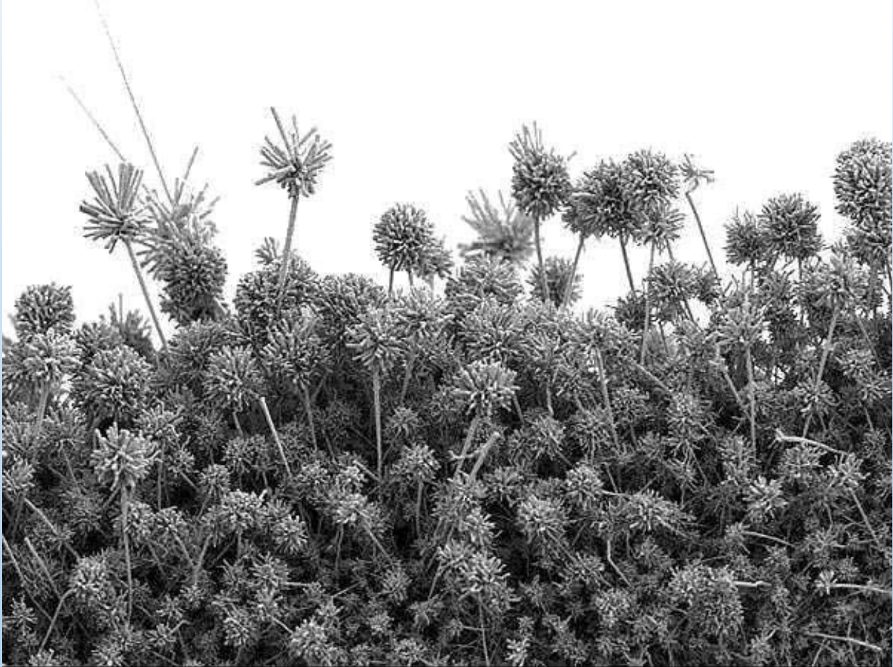
Chemical vapor deposited copper oxide---5kV---100X courtesy of Jim Stets, Air Products Co.
