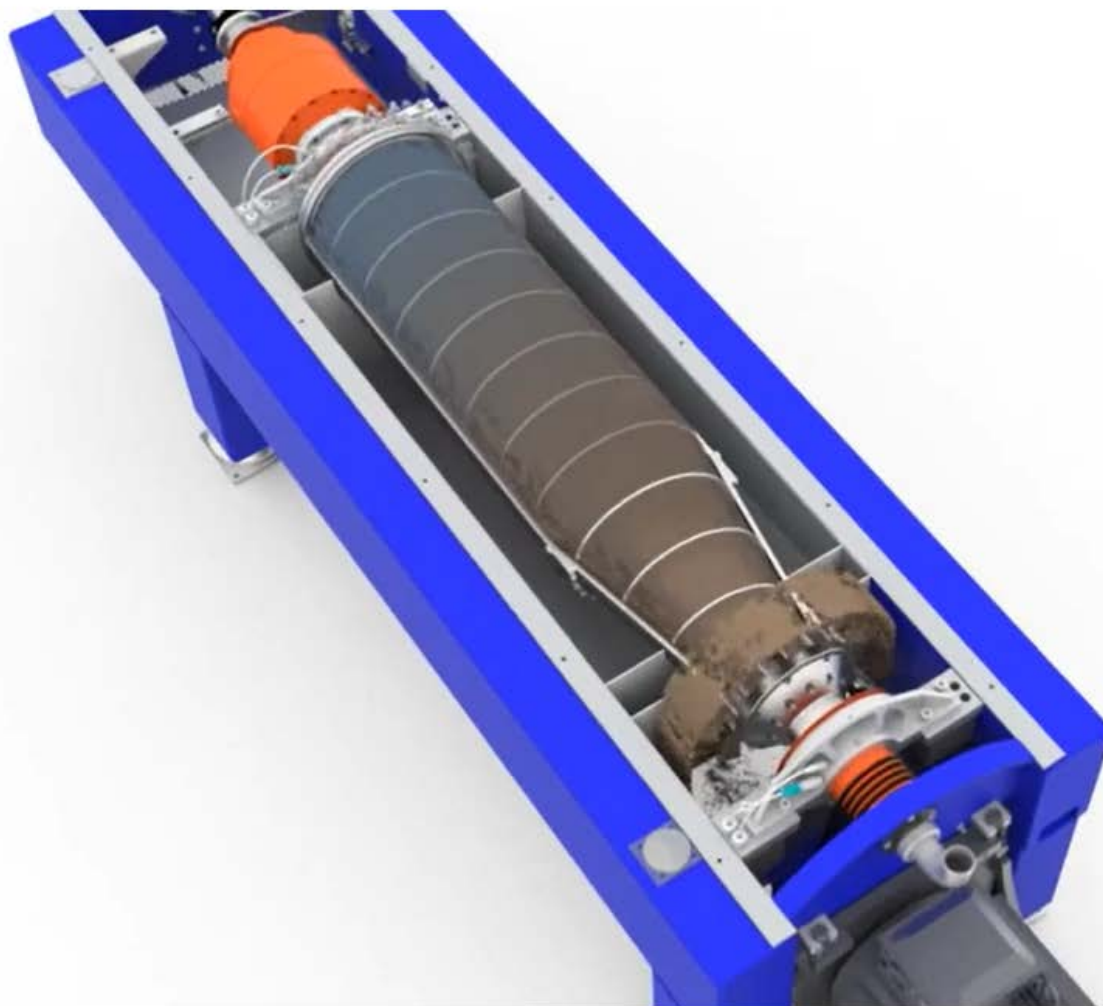
Animation | Alfa Laval wastewater treatment decanter centrifuge for sludge thickening and dewatering
