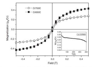
Figure 5. Magnetization versus magnetic field at 300 K for Cr:  $TiO_2$  films grown on an Si substrate at 650°C and 700°C. The inset shows the M(T) curve taken under 0.2 T for the film fabricated at 700°C.
