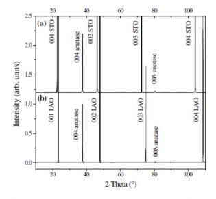
Figure 1. X-ray diffraction pattern (a) for a Co:TiO<sub>2</sub> film on STO under oxygen pressure of  $1 \times 10^{-5}$  Torr and fluence of 3 J cm<sup>-2</sup> and (b) for a Co:TiO<sub>2</sub> film on LAO under oxygen pressure of  $1 \times 10^{-6}$  Torr and fluence of 1.5 J cm<sup>-2</sup>.
