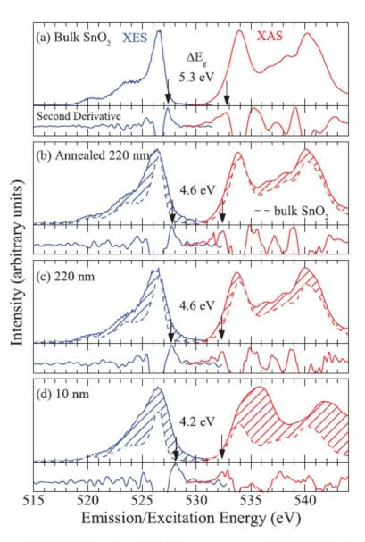
FIG. 3. (Color online) O K-edge x-ray emission (O K $\alpha$  XES) and absorption (O 1s XAS) spectra for bulk SnO<sub>2</sub> (a), the 200-nm-thick SnO<sub>2</sub> thin film with postannealing treatment (b), the 200-nm-thick as-grown film (c), and the 10-nm-thick as-grown film.
