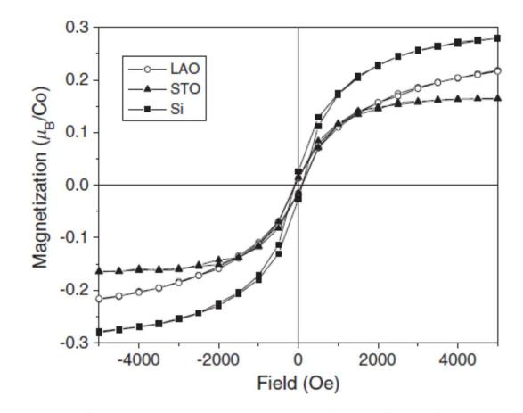
Figure 2. Magnetization versus magnetic field at 300 K for the  $\text{Co}: \text{TiO}_2$  film fabricated at 700°C, under an oxygen pressure of  $10^{-6}$  Torr on Si, LAO and STO substrates.
