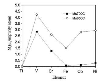
FIG. 8. Saturation magnetization vs element for TM: TiO<sub>2</sub> films fabricated at 700 and 650 °C {quantitative data taken from the saturated magnetic moments deduced from [M(H)] curves measured at 300 K}.
