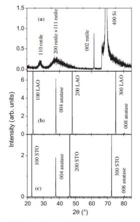
**Figure 1.** XRD pattern for a Co : TiO<sub>2</sub> film deposited at 700°C (*a*) on a Si substrate, under an oxygen pressure of  $10^{-5}$  Torr; (*b*) on a LAO substrate under an oxygen pressure of  $10^{-6}$  Torr and (*c*) on a STO substrate under an oxygen pressure of  $10^{-5}$  Torr.
