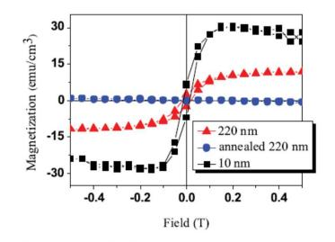
FIG. 2. (Color online) Magnetization versus magnetic field taken at 300 K as the magnetic field is applied parallel to the film's plane for the as-grown 10-nm-thick  $SnO_2$  film, the as-deposited 220-nm-thick  $SnO_2$  film, and the 220-nm-thick  $SnO_2$  film postannealed under the  $O_2$  atmosphere of 760 Torr at 700 °C for 10 hours.
