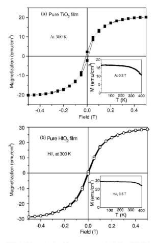
FIG. 1. Magnetization (a) versus magnetic field at 300 K for a pure TiO<sub>2</sub> film grown on a LAO substrate. The inset shows the M-T curve taken at 0.2 T and (b) versus magnetic field at 300 K for a pure HfO<sub>2</sub> film grown on an YSZ substrate. The inset shows the M-T curve taken at 0.5 T. (Note that the signals of substrates were subtracted already.)
