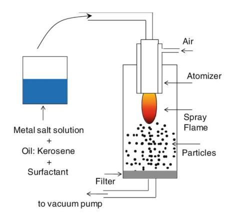
During the Flame combustion process, size of nanoparticles can be controlled by means of:
