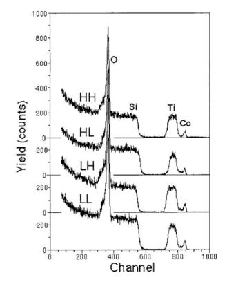
FIG. 4. RBS spectra of Co-doped  $TiO_2$  films with four different conditions: (a) LL, (b) LH, (c) HL, and (d) HH.
