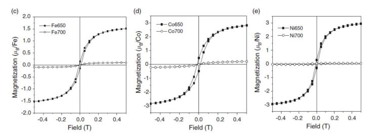
Figure 7. Magnetization versus magnetic field at 300 K for TM : TiO<sub>2</sub> films grown on LAO substrates at 650°C and 700°C: (*a*) V : TiO<sub>2</sub>, (*b*) Cr : TiO<sub>2</sub>, (*c*) Fe : TiO<sub>2</sub>, (*d*) Co : TiO<sub>2</sub> and (*e*) Ni : TiO<sub>2</sub>.
