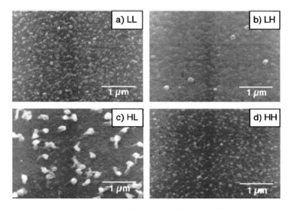
FIG. 3. SEM images of Co-doped TiO<sub>2</sub> films with four different conditions: (a) LL ( $P_{O_2}$  of  $1 \times 10^{-6}$  Torr and fluence of 1.5 J/cm<sup>2</sup>), (b) LH ( $1 \times 10^{-6}$  Torr, 3 J/cm<sup>2</sup>), (c) HL ( $1 \times 10^{-5}$  Torr, 1.5 J/cm<sup>2</sup>), and (d) HH ( $1 \times 10^{-5}$  Torr, 3 J/cm<sup>2</sup>).
