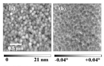
**Figure 6.** The topographic (*a*) and MFM (*b*) images obtained at room temperature on an area  $2 \times 2 \mu m^2$  of the V : TiO<sub>2</sub> film grown on Si at 650°C. The tip was applied perpendicular to the film's plane.
