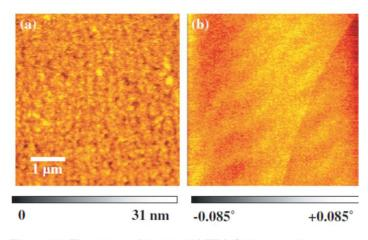
Figure 10. The topographic (a) and MFM (b) images taken at room temperature on the area  $5 \times 5 \,\mu \text{m}^2$  of the V : TiO<sub>2</sub> film grown on LAO at 650°C. The tip was applied perpendicular to the film's plane: (This figure is in colour only in the electronic version)
