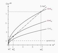
Equation has two, one, or no solution according to the value of  $C(\dot{m}_r)$ .
