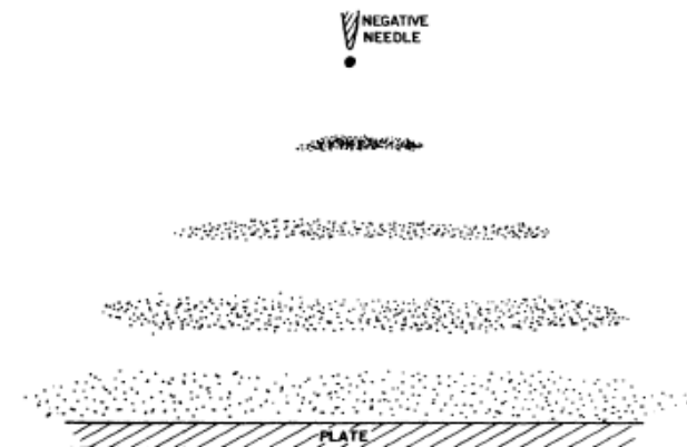
Fig. 8. Qualitative visual representation of our conception of spreading of negative ion cloud in transit across the gap at some voltage above threshold and below sparking. Spreading of charge cloud is due to Coulomb self-repulsion and spatial divergence of applied electric field. Diagram may also represent multiple charge clouds in gap at given time.
