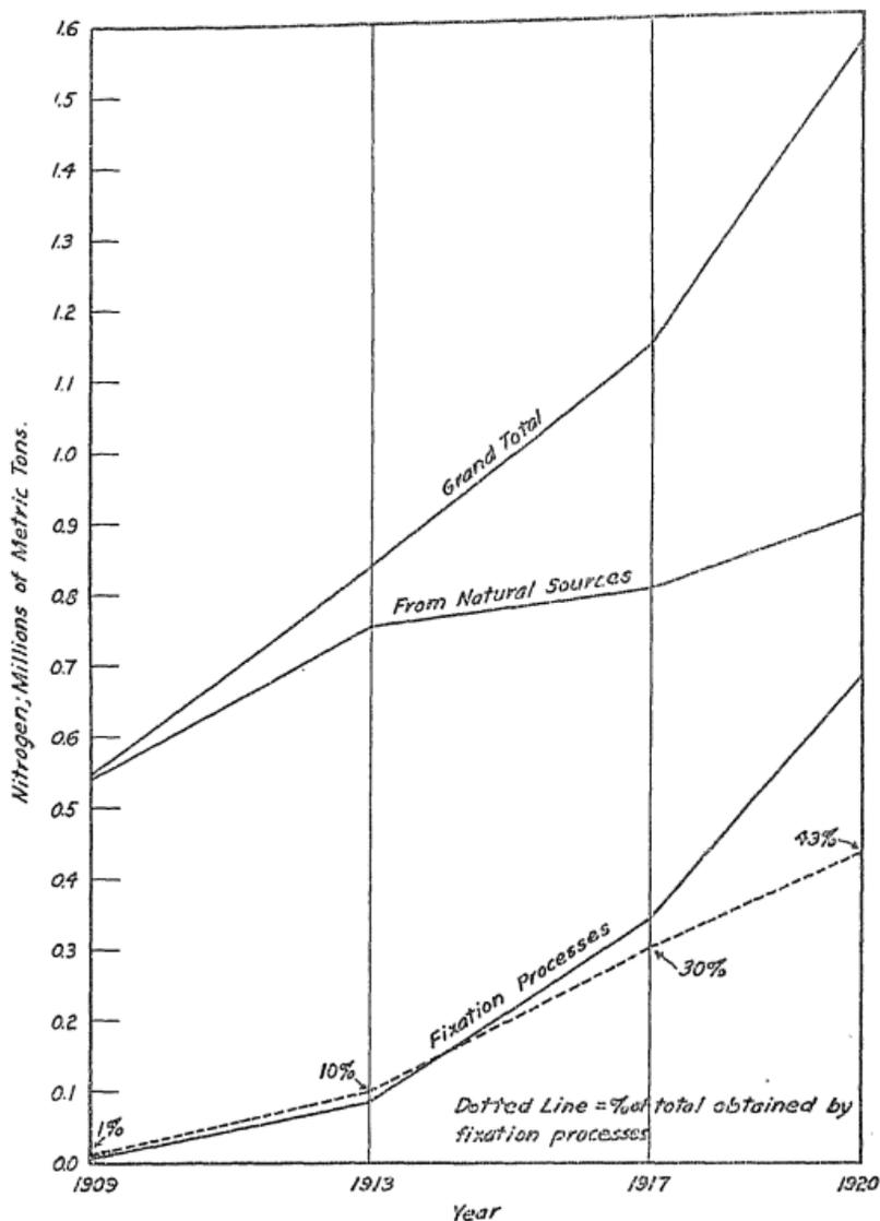
FIG. 51. THE RISE OF THE FIXED NITROGEN INDUSTRY
