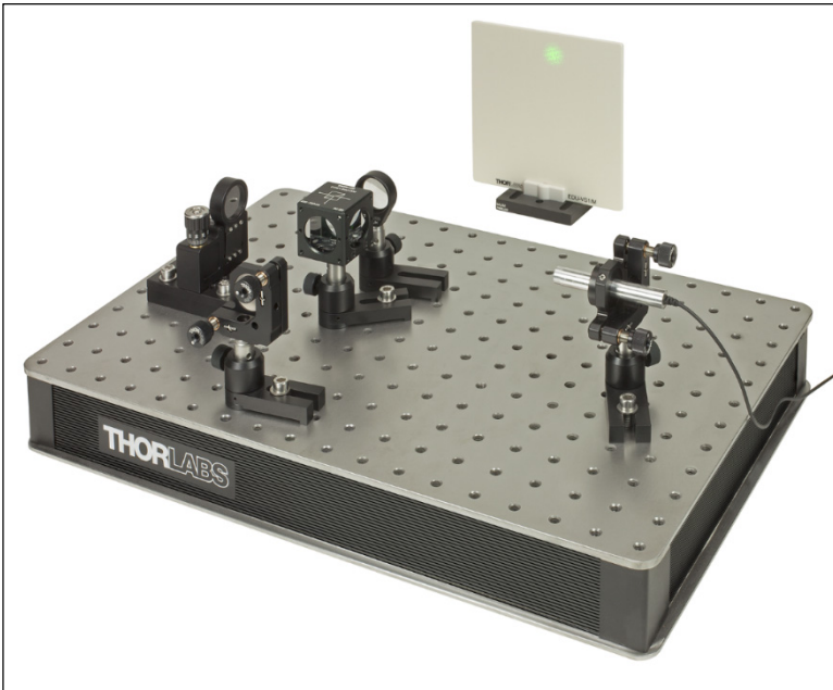
Figure 6 Alternative Placement of the Lens to Observe Lines
