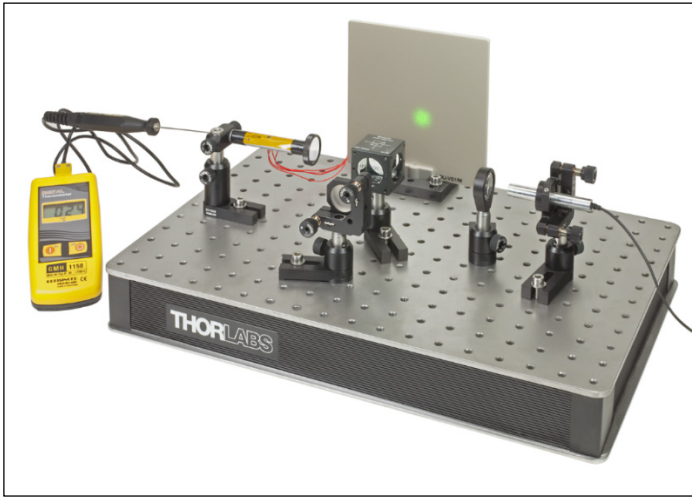
Figure 23 Setup to Determine the Coefficient of Thermal Expansion
