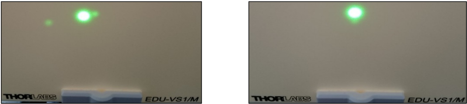
Figure 3 Laser spots with misaligned (left) and aligned (right) beamsplitter.
