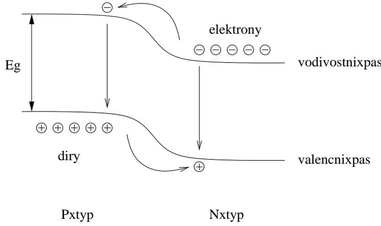
The width of the forbidden band is directly related to the photon energy of the emitted light and to the voltammetric characteristics of the diode, which brings a correlation between these two characteristics of the LED. We now discuss this relationship quantitatively and show how it can be used to approximate the value of Planck's constant.
