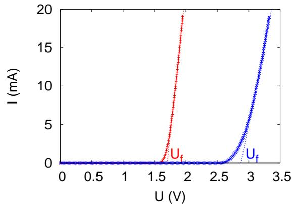
Obrázek 1: V-A characteristics of the red and blue LEDs with the voltage  $U_f$  indicated.
