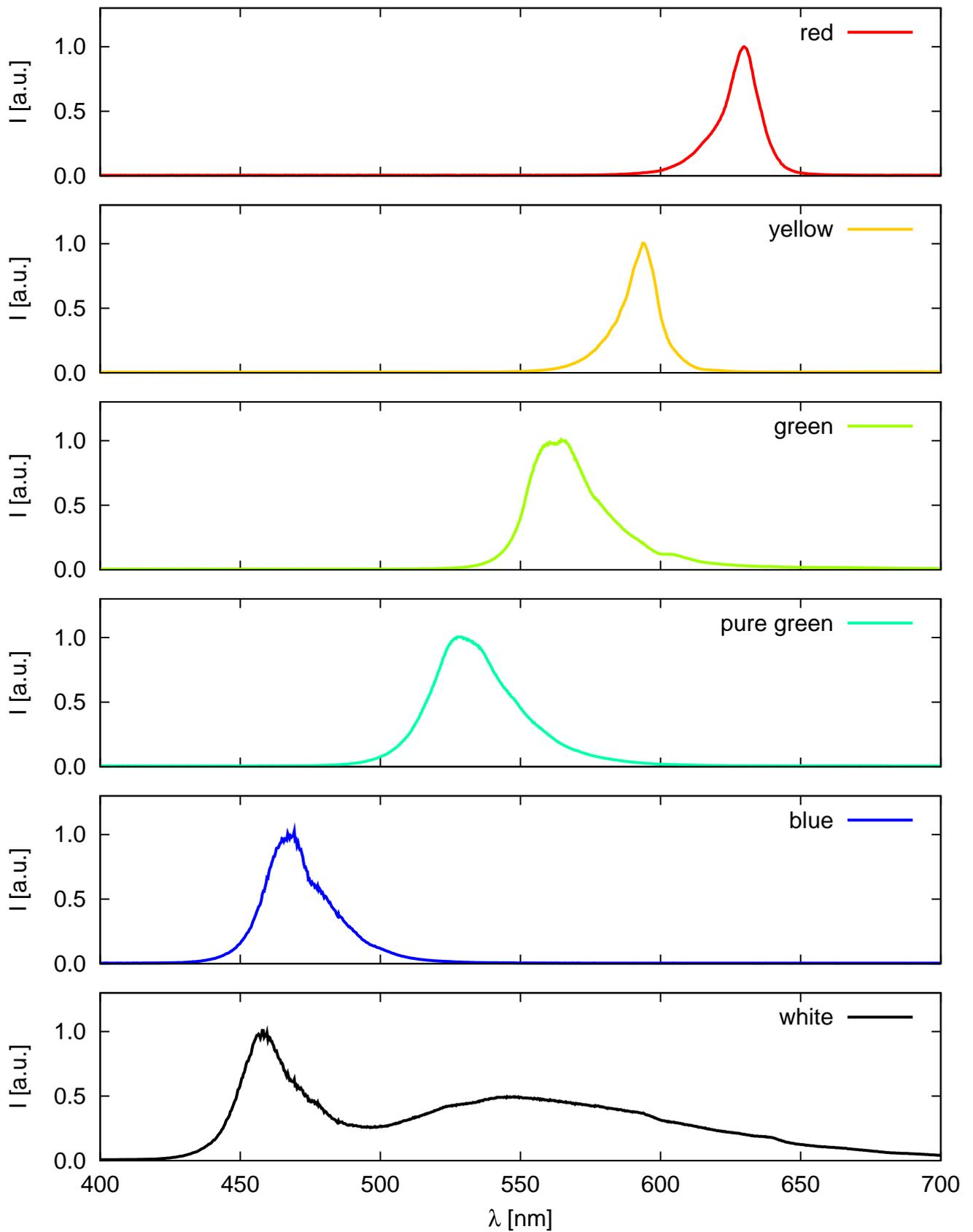
Obrázek 2: Emission spectra of LEDs of different colors available in practice. For LEDs labeled „white“ and „pure green“ intrinsic PN transition at wavelengths in the blue to UV region and the resulting color is achieved by phosphorescence.
