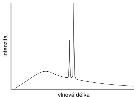
Obrázek 4: Spectrum of X-rays as the sum of the continuous and characteristic spectra.
