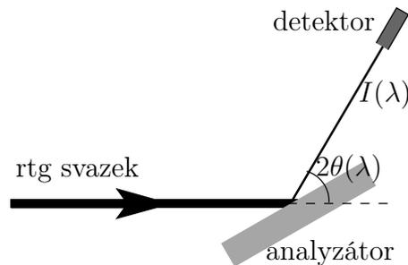
Obrázek 5: Scheme of an energy-sensitive measurement with a crystal analyzer.
