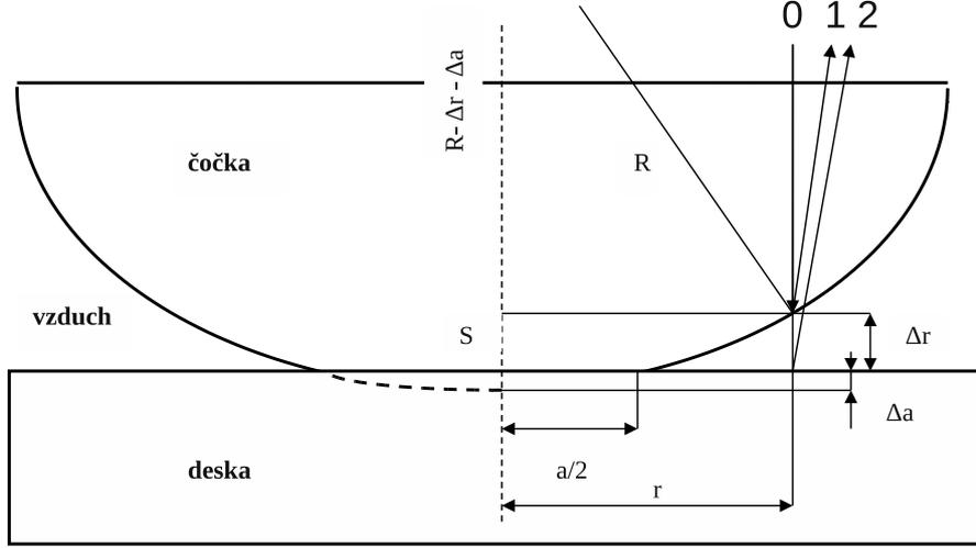
Obrázek 3: Schematic drawing of interfering rays on Newton's glasses.
