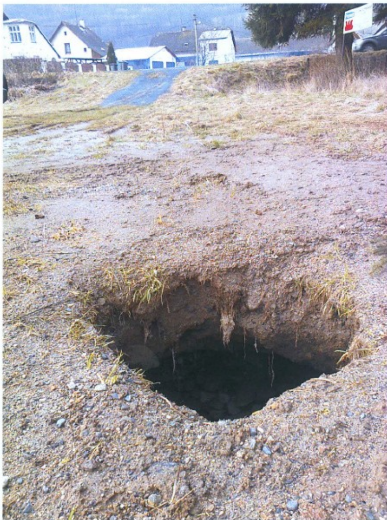
Obr. 1. Nedovrtný vrt 6432_6h s propadlou kavernou. Fig. 1. Unfinished borehole 6432_6h with collapsed cavern.
