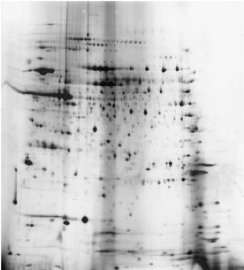
Figure 3. 2-DE spot pattern of proteins from phage 812; pH gradient 3–10; MS-incompatible silver staining.
