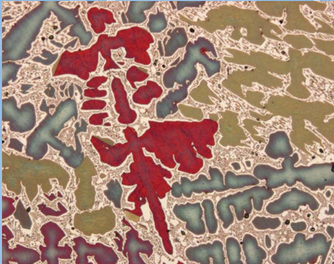
A micrograph of bronze revealing a cast dendritic structure
