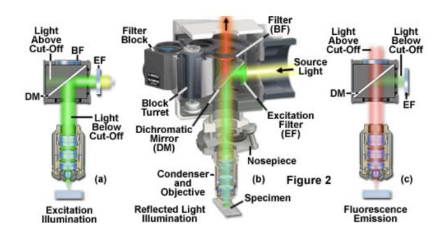
Dichroic mirror reflect light with lower wavelengths but transmit longer wavelengths. Thus, dichroic mirror reflects maximum of excitation light let go through maximum of emission light used for a particular fluorophore.
