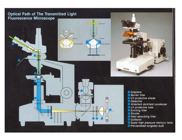
Excitation light goes through excitation filter and comes from below as in case of a classical wide-field microscope. The most important part here is darkfield condenser that adjusts excitation light path so the light illuminate specimen from sides. Thus, only fluorescence emission goes in objective and is observed through objective. Excitation light is reflected so does not enter objective.
