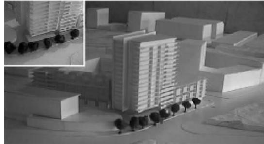
**Fig. 6: Photographs of the model of the Waterloo, Sydney development in Windtech Consultants' wind tunnel showing details of the optimum treatment for the effect of the westerly winds on the wind conditions at the north-western corner<sup>1</sup>**
