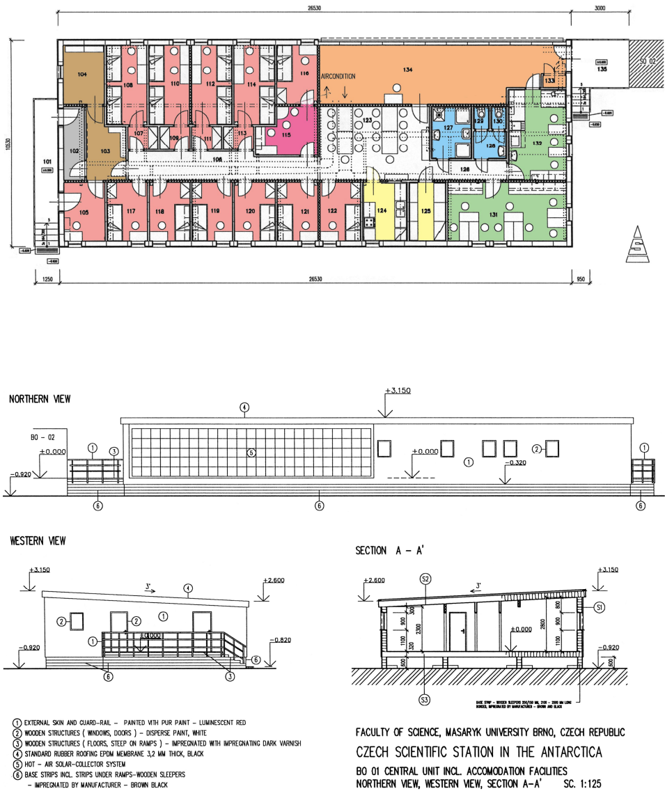
Fig. 5. Technical scheme of the main station building. View from the top shows entrance rooms (indicated in grey and brown), one- and two-bed rooms (pink), radio operator room (deep pink), central corridor and meeting room (white), kitchen and store room (yellow), laboratories (green), bathroom and lavatory (blue), workshop and hot air accumulation room (orange). Side view shows location of hot air collectors.
