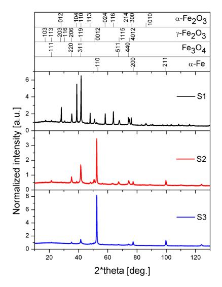
Fig.2 XRD patterns of the synthesised samples for three different gas mixtures. Dominant orientations for relevant iron and iron oxide allomorphs are shown, too
