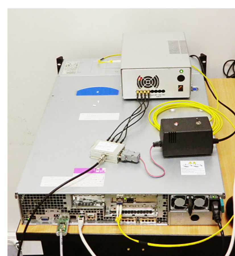
Figure 3: The preamplifier (in the front), the fast digitizer (in the back), and the measuring server (in the bottom).
