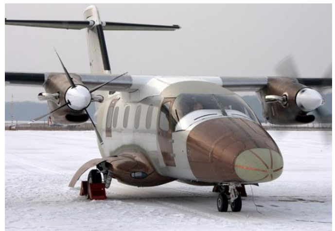
Fig. 2 Lightning diverters on EV-55.
