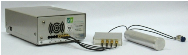
Fig. 2. Two parametric digital spectrometer. From the right: detector, amplifier with one input and two branches with different amplification, digital spectrometer.
