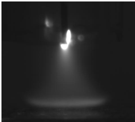
Fig.2. Image of the plasma needle glow.
