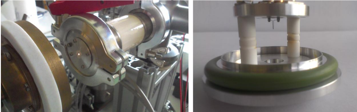
Fig. 2 Left: Image of transparent 100 nm stick window, when filament is heated, Right: Image of vacuum part of electron gun.
