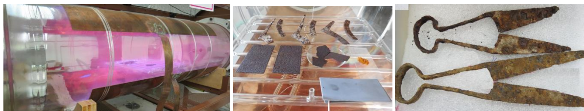
Fig. 1. Plasma reactor, model samples treated in plasma, example of treated object.
