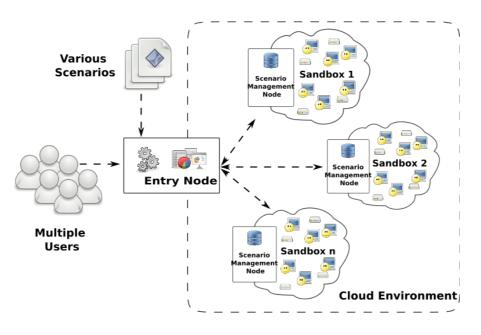
Figure 2: Caption: KYPO architecture schema. Users can access sandboxes via one entry node.
