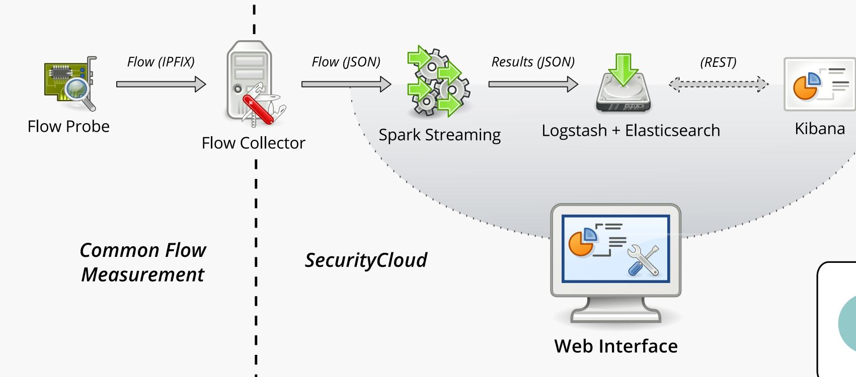
The demonstration cluster consists of 7 virtual machines, one is dedicated to IPFIXcol, 5 to Spark and one to the Kibana and Web server. The following configuration is the same for all machines:
