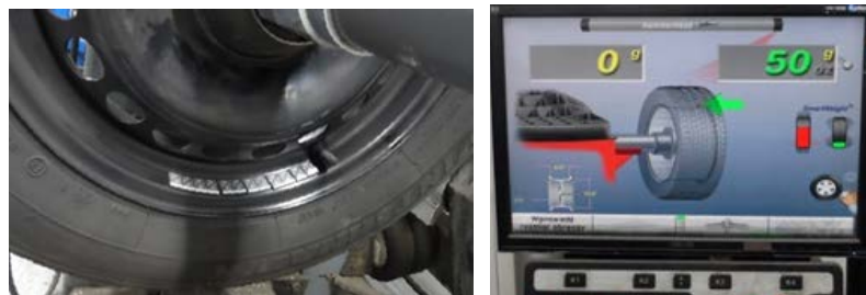
Fig. 4 – View how to place weights on the rim to the wheel unbalance and a view of the computer screen devices Hunter GSP 9700
