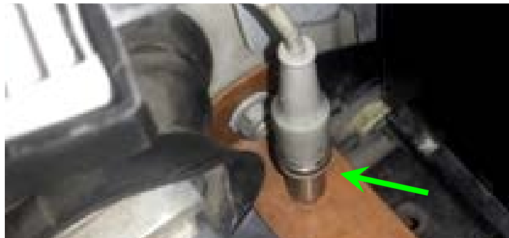
Fig. 2 – The view of where and how to place acceleration sensor on the car body above front right wheel suspension. Sensor indicated by green arrow
