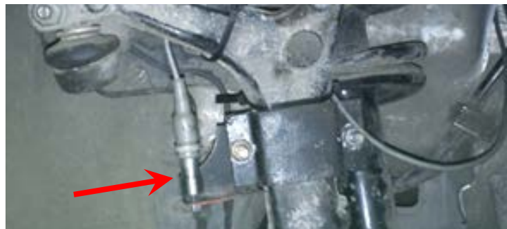
Fig. 1 – The view of where and how to place acceleration sensor on the front right suspension stub axle. Sensor indicated by red arrow
