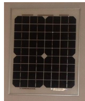
Figure 2: Monocrystalline solar panel
