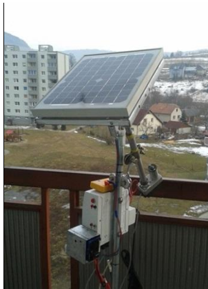
Figure 3: Dual – axis tracker system
