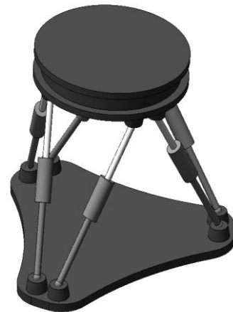
Figure 2: Schematic CAD model of the hexapod
