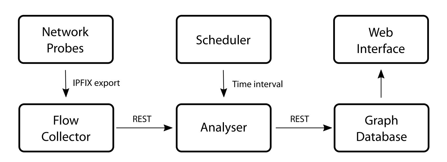
**Scheduler** – controlling component which invokes data analysis. It is important to schedule the analysis to match collector data storage interval so that each run of analysis has new data to process.
