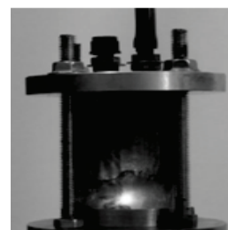
Figure 2. Photo of a discharge in n -heptane.
