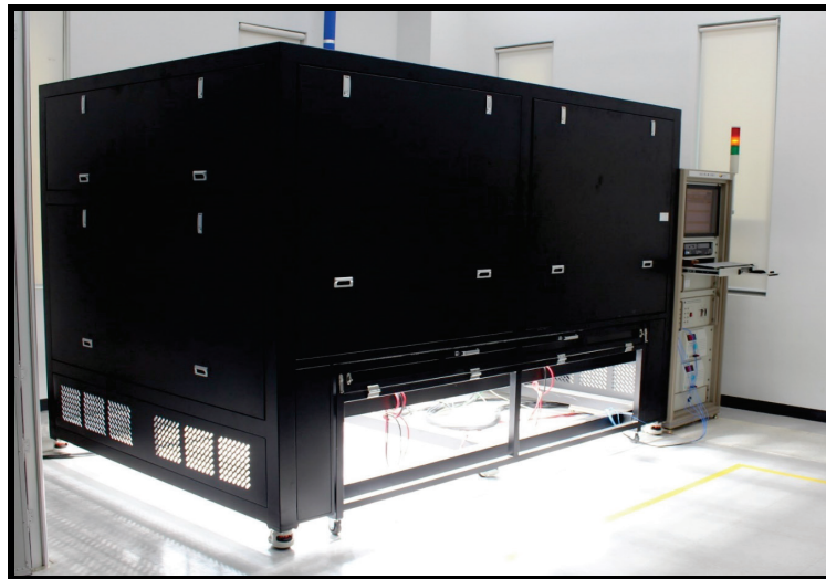
Figure 8. A solar simulator using 16 units of SolaRay plasma lights with the total power of 16 kW. It is used to inspect a large solar panel for its performance quality. SolaRay is the best light source for such an application owing to its near perfect spectrum close to the sun light. SolaRay lights were classified as a Class AAA light source for solar simulations. [Courtesy Woowon Tech in Seoul].
