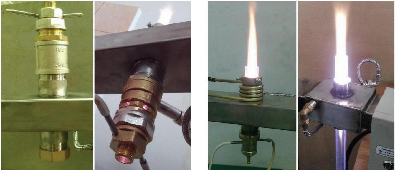
Figure 2. Plasma jet on standard fittings (left) and additional water cooling.
