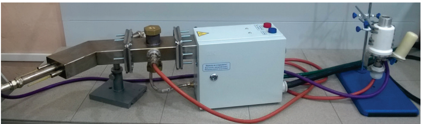
Figure 1. Atmospheric pressure microwave plasmatron installation.
