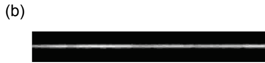
Figure 6. (a) Length of the plasma as a function of microwave pulse duty ratio. Peak microwave power is 1 kW and Slot width is varied from 0.1. To 0.7 mm. (b) High-speed camera image of the plasma at a peak microwave power of 2 kW and a duty ratio of 92%.
