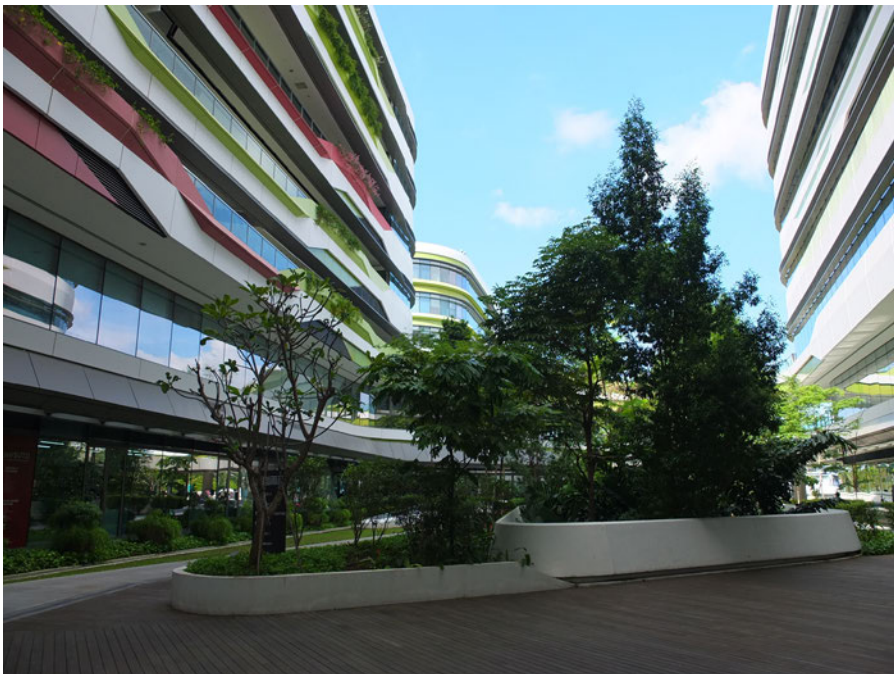
Figure 5.25 Contrasting materials help to identify edges between path and adjacent area, Singapore University of Technology and Design, designed by UNstudio (Photo by Z. Čerešňová)
