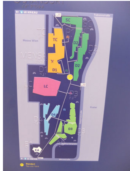
Figure 4.3 Tactile orientation plan with Braille and embossed lettering, WU campus in Vienna (photo: Z. Čerešňová)
