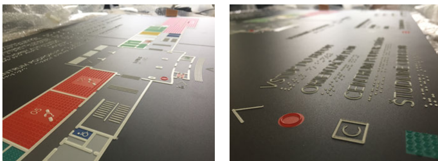
Figure 5.28 a, b Details of the tactile floor plan of the Faculty of Architecture, Slovak University of Technology in Bratislava (Photo by A. Kubica)
