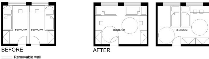
Figure 4.7 Example of spatial adaptability and flexibility – furniture can be arranged in rooms according to the individual needs of the user (source: L. Rollová)
